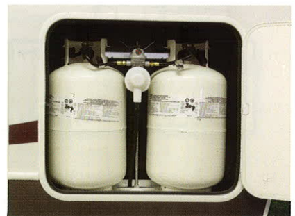
■ Easily accessible 30 lb. propane gas cylinders with auto changeover, and at the right height. No bending over!
