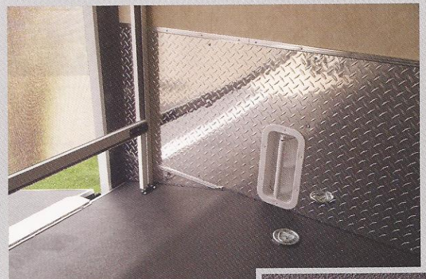
Track Mounted Roll Down Insect Screen, Side Wall Mounted Venting, Side Wall Diamond Plate, Dove Tail Rear Ramp Entry Detail with Tuff Ply Coating and 9 Tie Down Rings.
