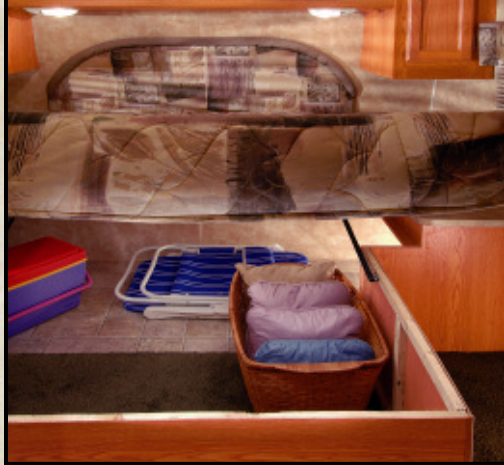
The walk around queen bed easily lifts up with the assistance of two gas struts to access another convenient large storage area .
