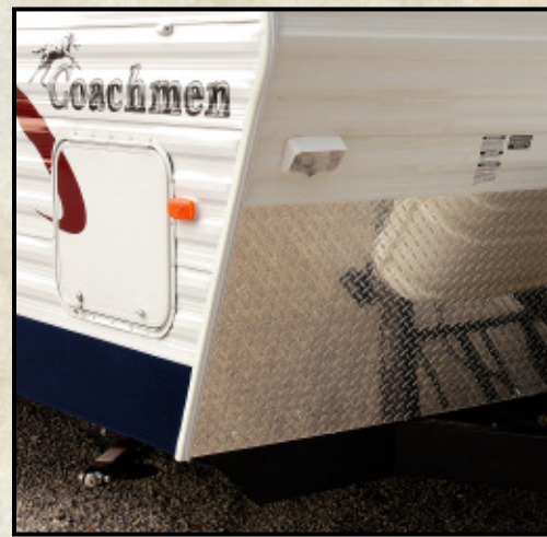
The diamond plate stone guard is a functional and attractive layer that is resistant to stone chips and other damage from road debris that you may come across in your travels. (Optional)
