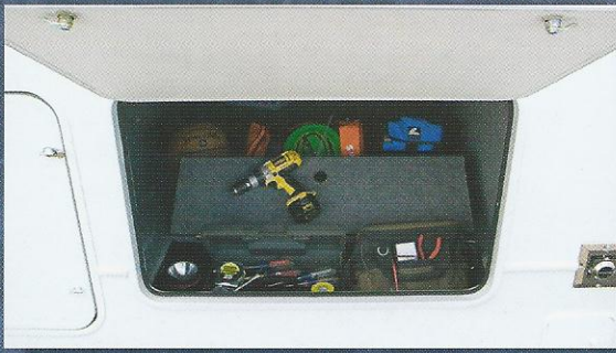
A steel toolbox with lid, recessed in the floor of the storage bay, is close to the door for easy access.
