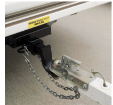
O The boat hitch doubles as a receiver hitch for a bicycle rack.
