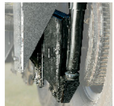
O The Mor/ryde (rubber independent suspension) system replaces the standard leaf spring suspension to provide smoother towing and better protects your RV from road shock.
