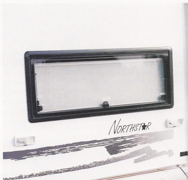
Insulated gas filled window. (Hardwall units only)
