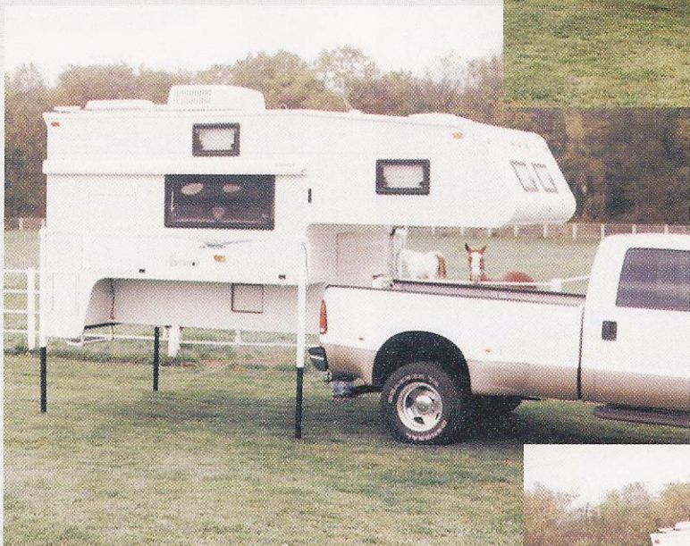
3. Line truck up and slowly back under camper.
