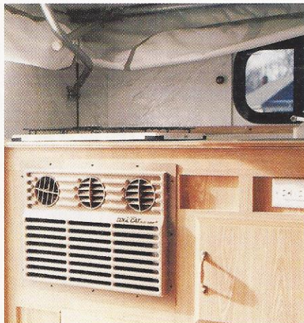
The All Electric Cool Cat Heat Pump provides 12,000 BTU's cooling and heat down to 40° ambient temperature. Note the clean appearance of canvas when in the down position.
