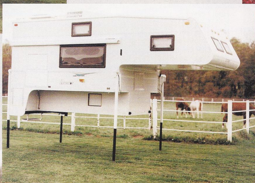
2. Raise until floor clears bed height.
