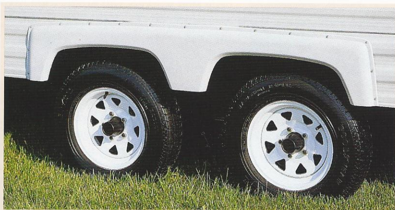
Radial tires are standard on all LITE Travel Trailers. Polyurethane wheel wells help provide an attractive finish. For improved ground clearance on some models, straight axles with 15" tires are optional.
