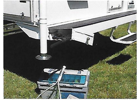
▲ Ranger's integrated bumper features a swing down step and handy, lockable storage.
