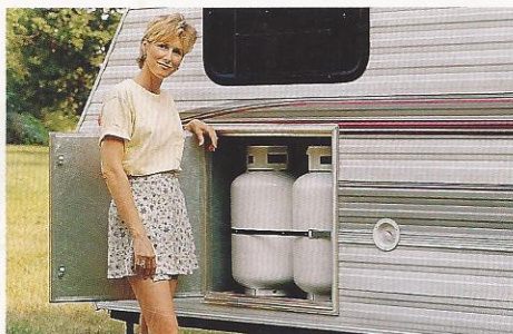
LP-gas bottles are stowed in their own easy-to-get-at compartment on the side of the RV.
