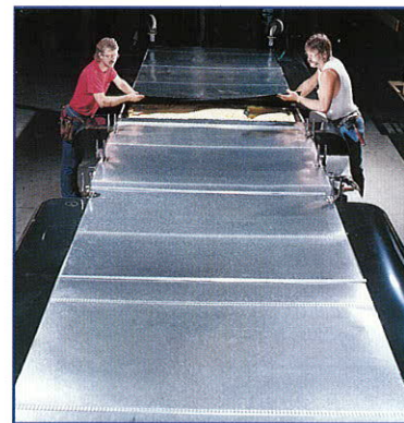
Completely Enclosed Metal Underbelly (No Plastic)
