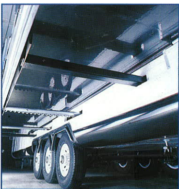
4 Season Insulation Package: R-19 Roof, Front & Rear; R-8 Sidewalls; R-26 Underbelly
