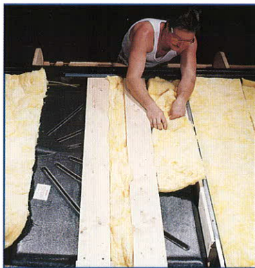
R-26 Fiberglass Insulation in Underbelly— Heated Holding Tanks
